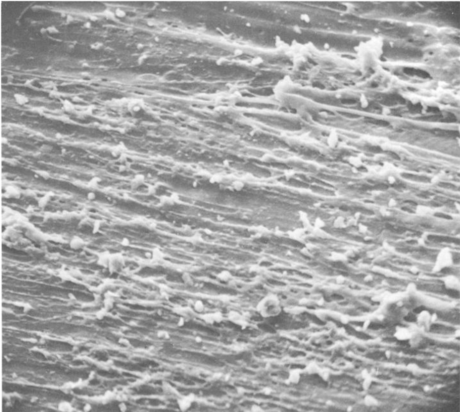
FIG. 2.—SEM photomicrograph of an exterior paint surface having an unusual topography; taken from a 1970 Chevrolet (400 \times ).
